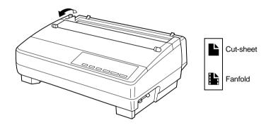
Grasping the two back corners of the printer with the palms of your hands, press back on the two raised areas on the top of the rear cover until it opens.
