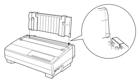
☐ To remove the paper guide from the printer, simply pull the tabs out of the holes.
