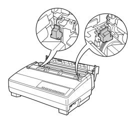
A piece of cardboard is inserted into the printer to protect components during shipping. Be sure to remove it before using the printer.
