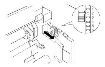
Move the adjustment lever to one of its six settings. Position 2 is most suitable for single-sheet paper.
