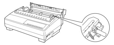
☐ Before printing, make sure that the leading edge of the fanfold paper extends about 0.8 inch (two centimeters) past the front the paper chute, as shown in the illustration below.
